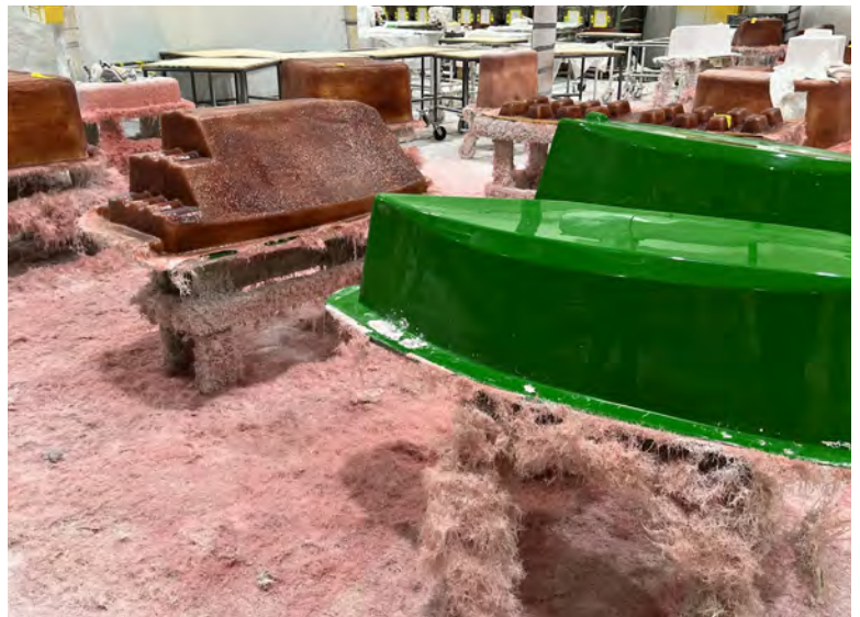
The messy process of fiber and resin sprayed onto a boat mold.
