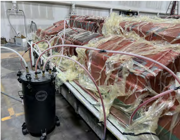
Vacuum-impregnation process with plastic bag vacuum sealed to mold.
