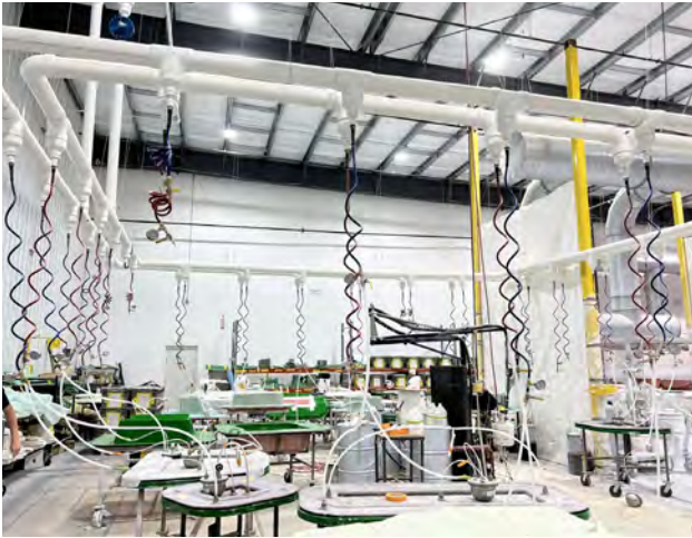
Fiberglass mat and resin placed on molds during vacuum-impregnation.
