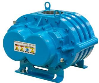
CP Series rotary blowers are designed to be interchangeable with equivalent sizes of competitive models. They are rated up to 18 PSIG discharge pressure or 16" Hg dry vacuum.
