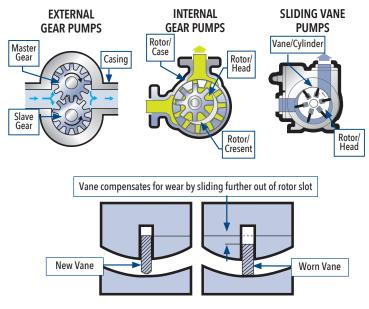
The clearances of a gear pump are tightest when it is taken out of the box, but then begin to degrade as soon as the pump is put into operation. Sliding vane pumps, on the other hand, suffer no clearance degradation because the vanes self-compensate for wear.
