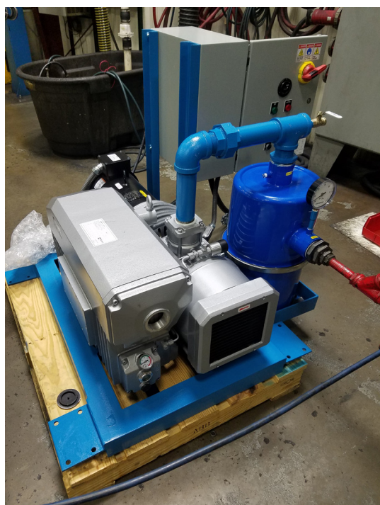
All-in-one mobile unit with control panel, Kinney KVA 250 pump and inlet knock-out pot.
