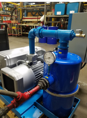
Separator tank with Kinney KVA 250 pump and motor.
