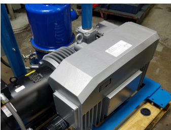
The heart of the package is the Kinney KVA 250 single stage, oil-sealed rotary vane vacuum pump.
