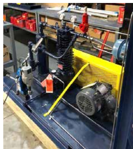
Blackmer heavy-duty compressor model HD082B mounted on structural steel baseplate.
