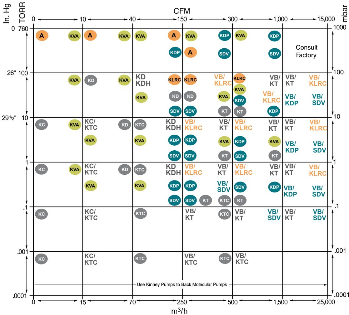
**Example:** For 50 CFM and 80 Torr, the selector guide indicates that KD, KDH, KVA, KLRC, KDP, and SDV pumps should be considered.
