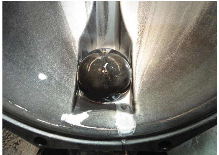
View of fluid end cap (Rotated 180°) where ball was pushed through seat into end cap.
