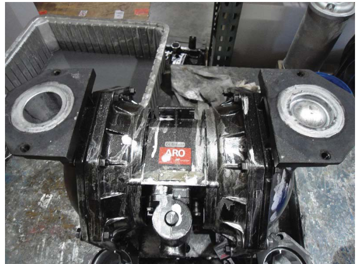
Pump view with discharge manifold removed showing right ball check pushed through seat into fluid end cap.
