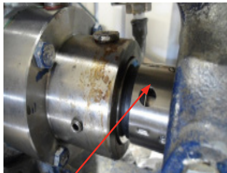
We custom designed a low operating height Type 8 mechanical seal in place of the lip seal for improved sealing.
