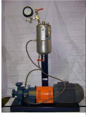
Dean pH2111 1x1.5x6 in 316ss construction 7.5hp EXP motor ASI model 595 double mechanical seal API Plan 53 barrier tank setup Custom pump base with seal pot stand to keep the package compact.
