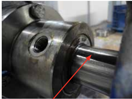
The original lip seal was installed in the back of the stuffing box to keep the oil inside the box.
