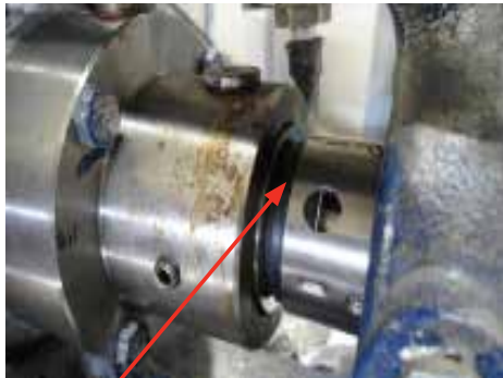
We custom designed a low operating height Type 8 mechanical seal in place of the lip seal for improved sealing.
