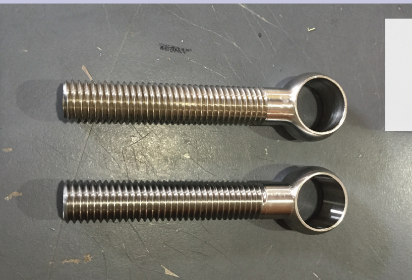
Original part – Top bolt Duplicate part – Bottom bolt
