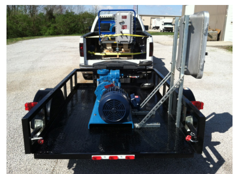
The excess deck space around the pump leaves room for operator safety when attaching hoses to the pump and storage space for hoses to stay with the package.
