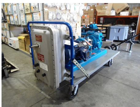
Similar to the trailer packages the pump and control panel for the cart are installed to maintain maneuverability and ease of use.
