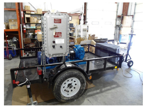
Once the pump is secured to the deck, bracing and supports are added to accommodate the control panel. A tongue storage box is also added to house wheel chocks and provide additional storage.
