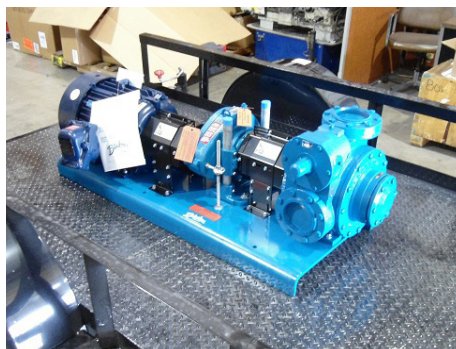
The pump is positioned on the trailer to keep the balance of the trailer and tongue weight as close as possible to its unloaded state.
