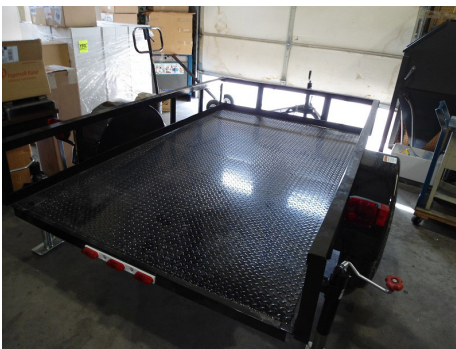
The treadplate steel floor gives us a solid base to start construction.
