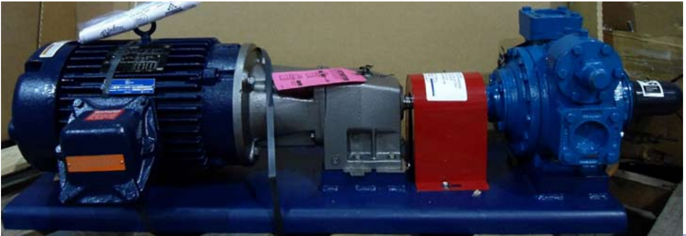
BlackmerSGL Series Ductile Iron Pump for refrigerants and other liquified gas service.
