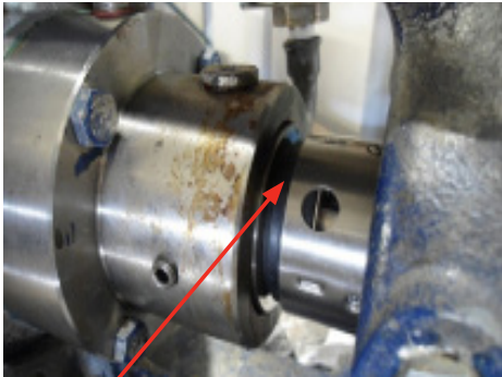
We custom designed a low operating height Type 8 mechanical seal in place of the lip seal for improved sealing.
